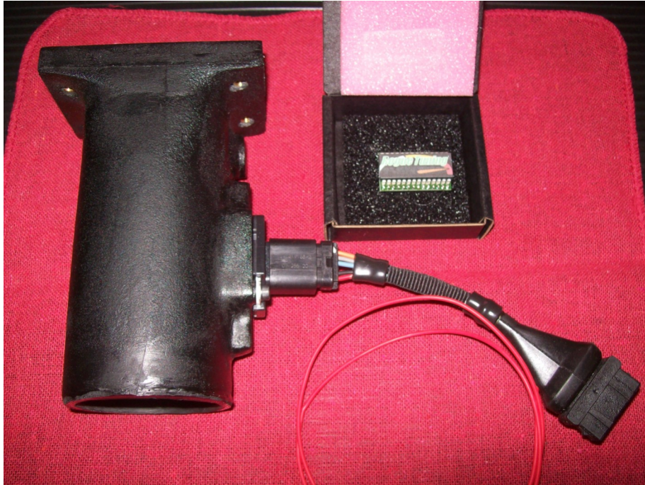
The NA-Tune Kit - The kit includes the MAF Assy and the Chip/Chip Board
