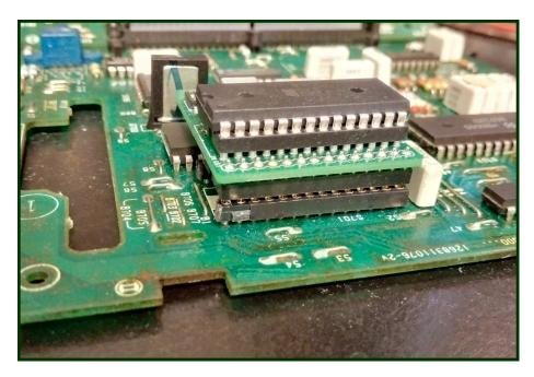
**Step 13** - Make sure the chip and chip board are fully seated as shown above.
