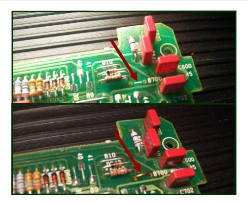
**Step 15** - Add the jumper wire as shown above. The jumper wire is soldered on the back side of the board.
