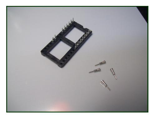
**Step 10** - Chip socket pins will need to be obtained and are readily available online in the form of individual pins or sockets (and then pins can be removed)
