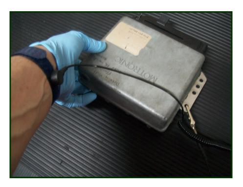
**Step 3** - When handling electronic equipment it is important to protect the components from ESD (electro-static discharge). An ESD wrist strap is recommended as shown above. These wrist straps are readily available online.
