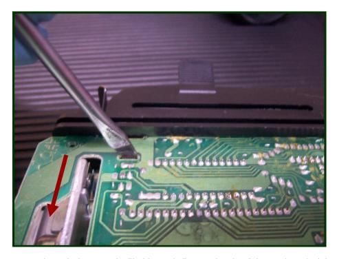
**Step 6** - Gently push down on the "holding tabs" on each side of the top board while pulling back on the board as shown above.
