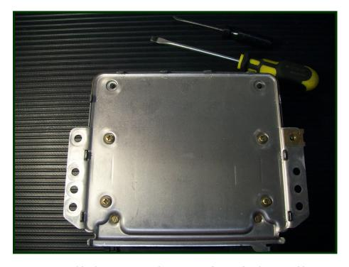
**Step 16** - Re-assemble the DME using the reverse of steps for dis-assembly.
