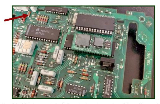
**Step 14** - Add a jumper wire in the location shown above. Step 15 shows close up details for the jumper wire.
