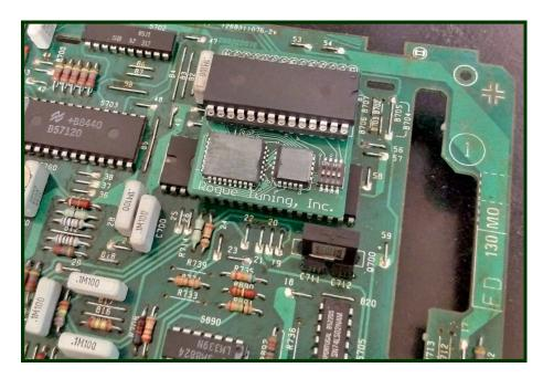
**Step 12** - Install the Rogue Tuning chip board as shown above. Notice the orientation of the chip board and make sure it is installed **EXACTLY** as shown.
