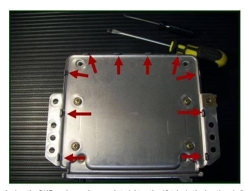
**Step 1** - Lay the DME as shown above and straighten the 10 tabs in the locations indicated.
