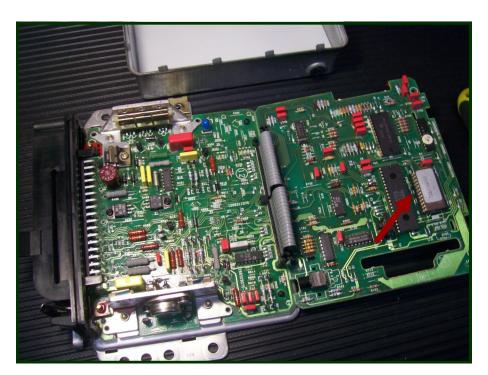
**Step 7** - Open up the printed circuit boards so that the components including the DME chip are exposed as shown above..
