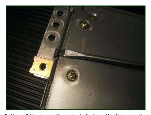
**Step 2** - Using a flat head screw driver, get under the tab and bend them straight up.
