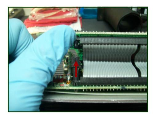
**Step 5** - Separate the printed circuit boards. Use your thumbs on both sides of the connector pushing up as shown to separate the connector posts that snap together.
