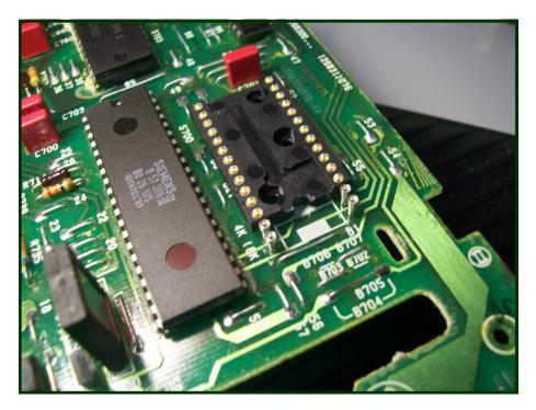
**Step 11** - Install the four additional socket pins. The pins are soldered on the back side of the board and need to be straight and level with the 24 pin socket as shown above.
