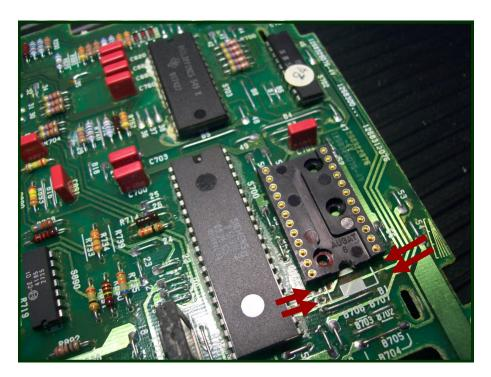
**Step 9** - With the chip removed we can see the four locations in which "chip pins" must be added as shown above.
