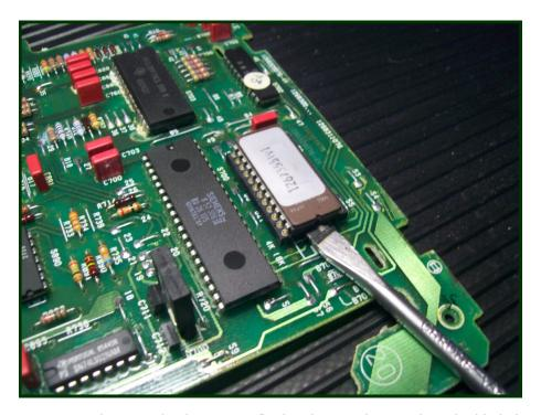
**Step 8** - Remove the DME chip by using a flat head screw driver. Place the blade beneath the chip at the socket and gently rotate the blade from side to side to work the chip out of the socket. Go back and forth between the two ends of the chip to bring the chip up as evenly as possible.
